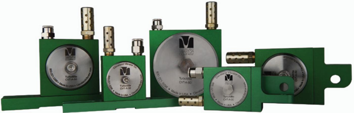
Fabricated with lightweight anodized aluminum, the unique body design of our Turbomite CVT-A Series Turbine Vibrators allows for multiple mounting foot bases with the same body. Our off-the-shelf mounting styles are designed to accommodate existing bolt-hole patterns from competitor turbine and ball vibrators. Or, use your own mounting to integrate our highly powerful and efficient turbine into your design.
