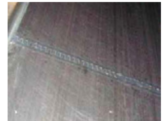
PVC splice in an airport belt
