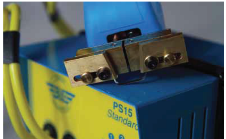
2 cap screws adjust the depth of the blade
